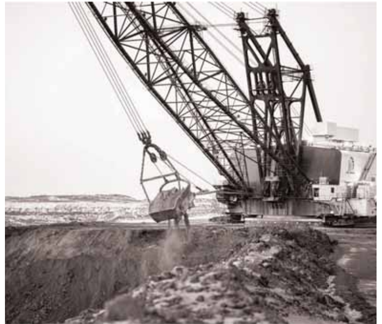
Submitted photo | North American Coal A dragline removes overburden at Falkirk Mine near Underwood, North Dakota.
