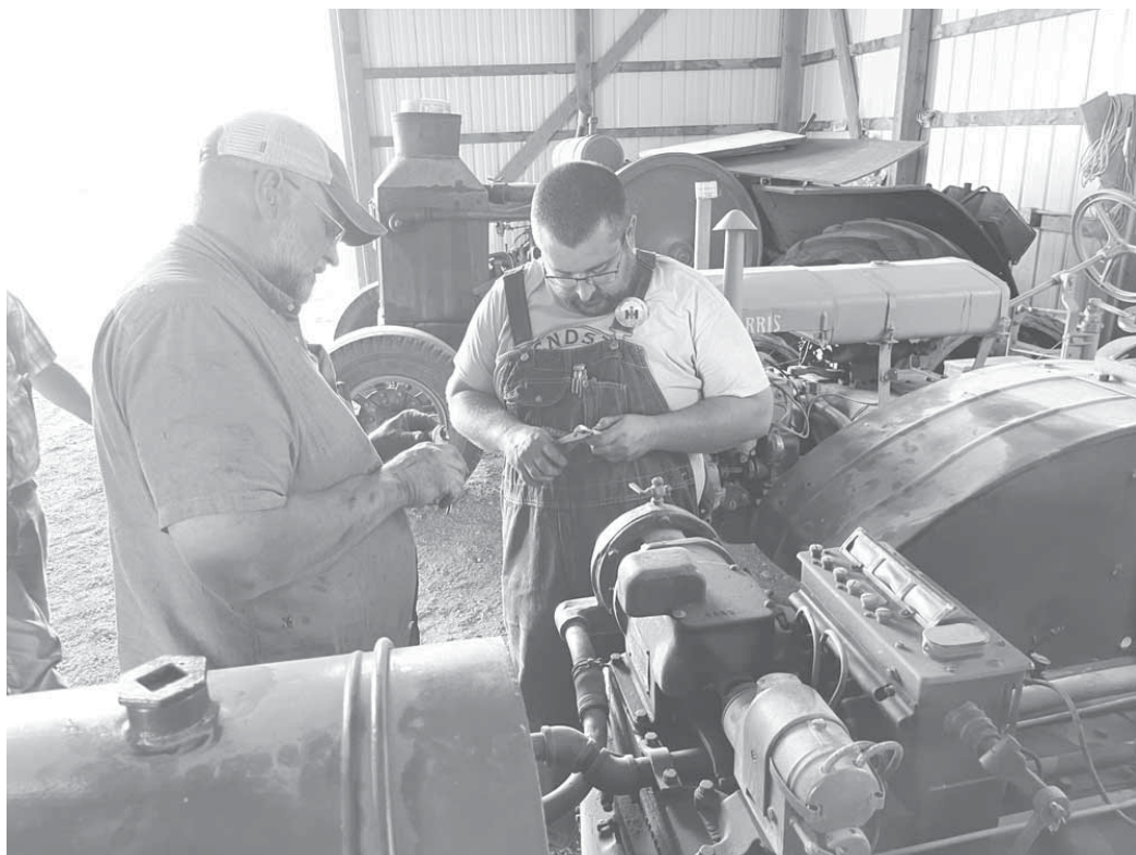
Dean Lemer and Chris Sisson cleaning spark plugs on the MTA’s Hart Parr 12-24. The tractor was Loren Quandt’s, and it hadn’t run since 2015.
