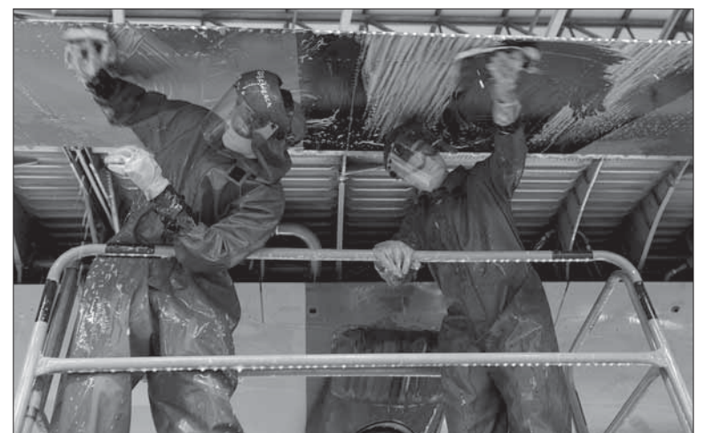
Airmen with the 86th Maintenance Squadron wash a wing of a C-130J Super Hercules before a C-2 isochronal inspection Jan. 4, 2016, at Ramstein Air Base, Germany. The examination marks the 14th and final C-2 ISO inspection for the 86th Airlift Wing until 2020. A C-2 ISO inspection lasts approximately two weeks and is an extensive examination of an aircraft to maintain its functionality and perform preventive maintenance.
