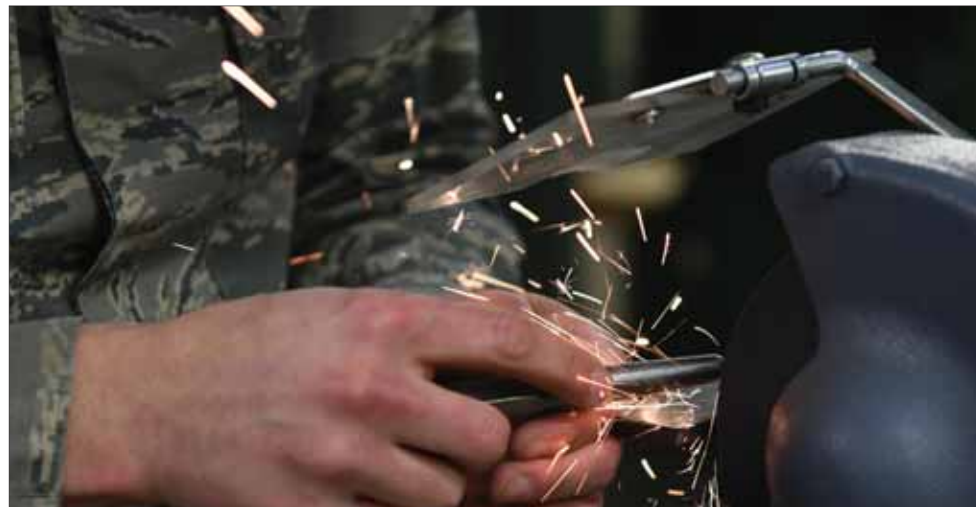
An Airman from the 5th Maintenance Squadron sheet metal shop dresses a center punch at Minot Air Force Base, North Dakota, Dec. 11, 2018. The center punch is a tool used for making indentations in metal to guide the drill correctly.
