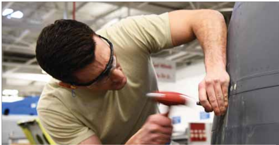
Senior Airman Joshua Sacerio, 5th Maintenance Squadron aircraft structural maintenance journeyman, uses a center punch at Minot Air Force Base, North Dakota, Dec. 11, 2018. A center punch is a tool used for making indentations in metal to guide the drill correctly.
