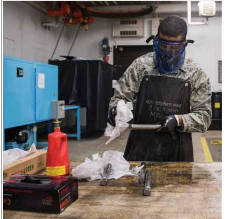
Airman 1st Class Marcus Watkins, 5th Maintenance Squadron non-destructive inspection apprentice, cleans iron particles off of a piece of equipment at Minot Air Force Base, North Dakota, Jan. 25, 2019. NDI technicians are responsible for identifying possible defects in systems and equipment before they become dangerous problems.
