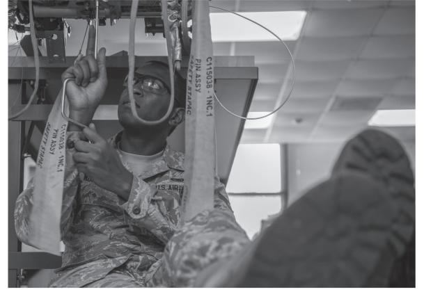
Senior Airman Sheldon Morrison, 7th Component Maintenance Squadron aircrew egress systems apprentice, attaches a pitch stabilization control assembly, or STAPAC, to a B-1B Lancer ejection seat at Dyess Air Force Base, Texas, June 26, 2019. The STAPAC controls the positioning of the seat upon ejecting with a rotating gyro, which allows the seat to remain upright. The 7th CMS egress shop was recently tasked to conduct an out-of-cycle inspection on all B-1Bs in Dyess' fleet.
