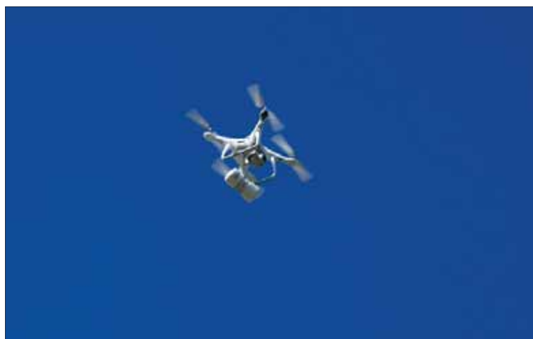
A drone simulates dropping a payload onto an improvised explosive device at Minot Air Force Base, North Dakota, Aug. 8, 2019. Airmen can safely trigger bombs by dropping a heavy object on an improvised explosive device.
