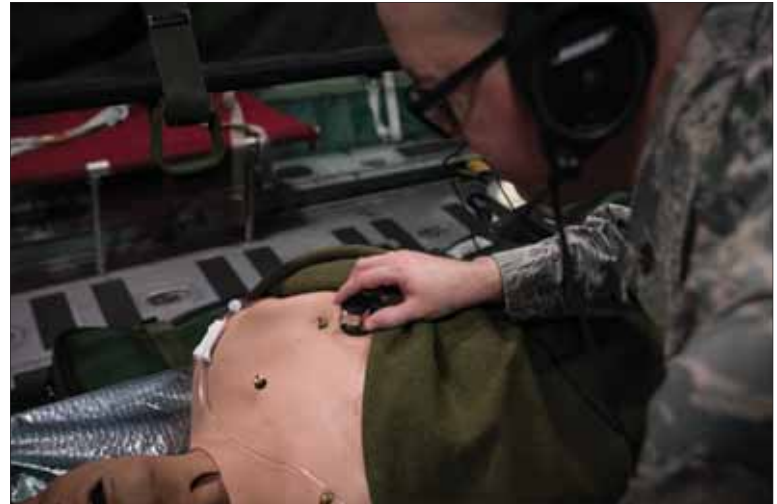
While testing the new wireless high-noise filtering stethoscope, Maj. Daniel Bevington, a nurse researcher in the 711th Human Performance Wing of the Air Force Research Laboratory, places the device on a mannequin's chest to listen to internal sounds.
