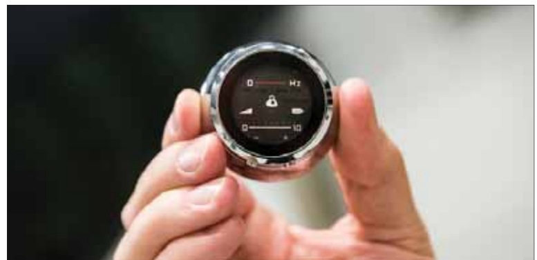
The new wireless high-noise filtering stethoscope that is being tested by researchers in the Air Force Research Laboratory's 711th Human Performance Wing, is displayed during a testing session. The device was developed by ThinkLabs.
