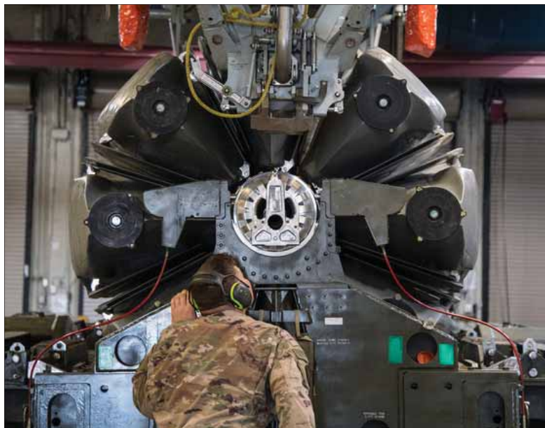
Senior Airman Ryan B. Jarvis, 2nd Munitions Squadron launcher maintenance technician, watches as the last Conventional Air-Launched Cruise Missile (CALCM) is loaded into a launcher at Barksdale Air Force Base, La., Nov. 20, 2019. The 2nd MUNS loaded the final CALCM missile package into a launcher in order to disassemble the weapon to become demilitarized.
