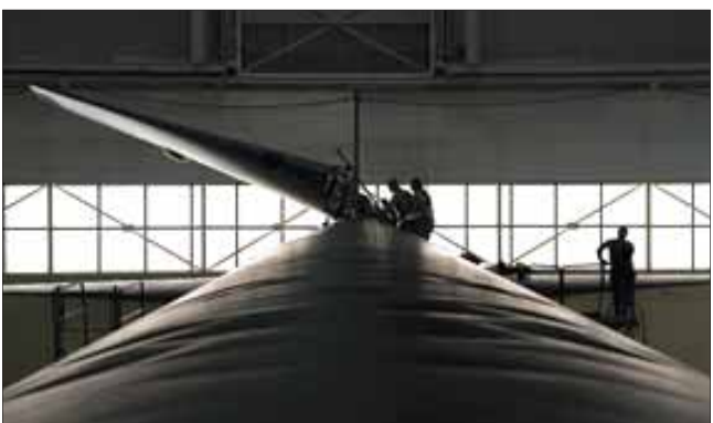
Crew chiefs assigned to the 5th Maintenance Squadron lower the vertical stabilizer on a B-52H Stratofortress at Minot Air Force Base, North Dakota, Feb. 10, 2019. Vertical Stabilizers are seldom taken down for maintenance.
