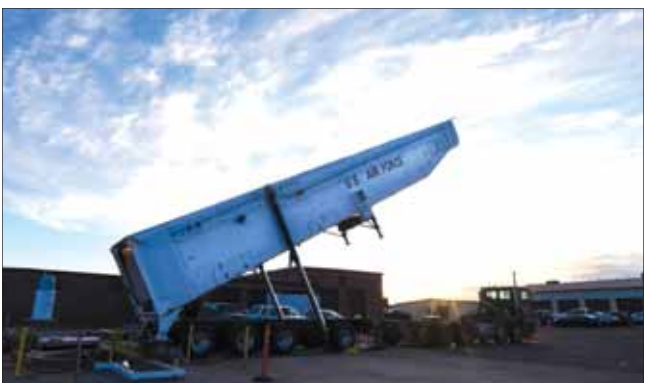
A transporter erector is raised during an annual proofload test at Minot Air Force Base, North Dakota, April 2, 2019. A transporter erector is used to downstage a Minuteman III intercontinental ballistic missile rocket engine into silos.
