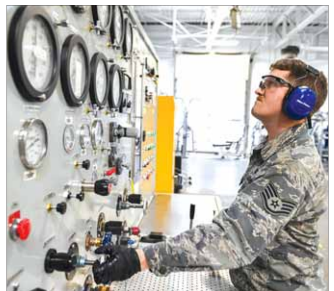
Staff Sgt. Stephen Foxworth, 5th Maintenance Squadron aircraft hydraulic systems craftsman, operates a hydraulic test stand at Minot Air Force Base, North Dakota, April 4, 2019. Aircraft hydraulic systems maintainers are responsible for ensuring aircraft hydraulic and pneumatic systems work properly.
