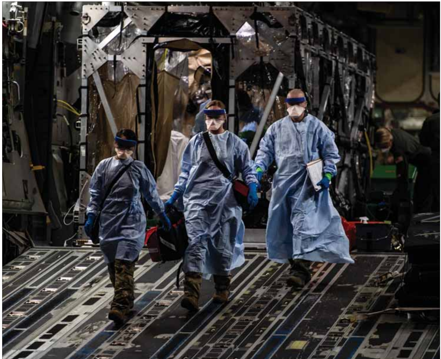
Three U.S. Air Force medical Airmen exit a C-17 Globemaster III following the first-ever operational use of the Transport Isolation System at Ramstein Air Base, Germany, April 10, 2020. The TIS is an infectious disease containment unit designed to minimize contamination risk to aircrew and medical attendants, while allowing in-flight medical care for patients afflicted by a disease—in this case, COVID-19. See story on page 2.
