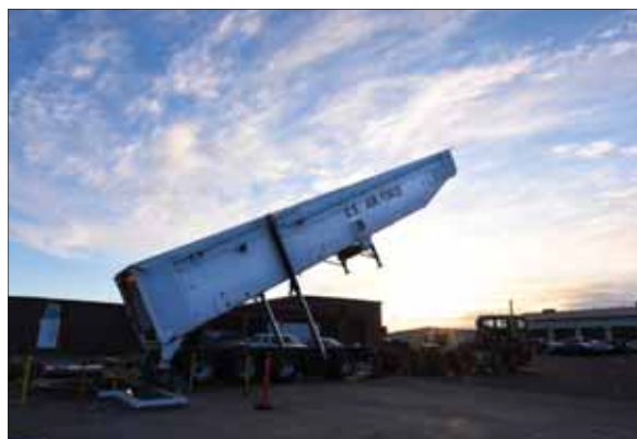
A transporter erector is raised during an annual proofload test at Minot Air Force Base, North Dakota, April 2, 2019. A transporter erector is used to downstage a Minuteman III intercontinental ballistic missile rocket engine into silos.
