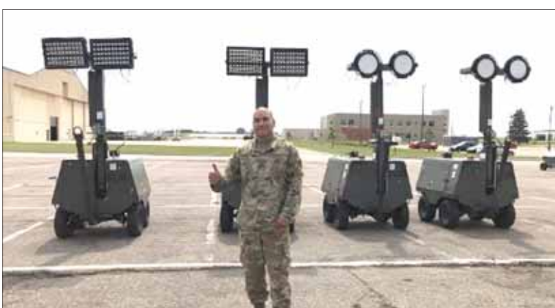
Air Force Global Strike Command 5th Maintenance Squadron AGE Section Chief, Master Sgt. Miguel Alvarez, in front of four flightline light carts retro-fitted with the two different Light Emitting Diode (LED) fixture options for testing.
