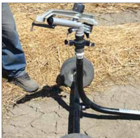
Golf course style sprinkler heads used for irrigation.
