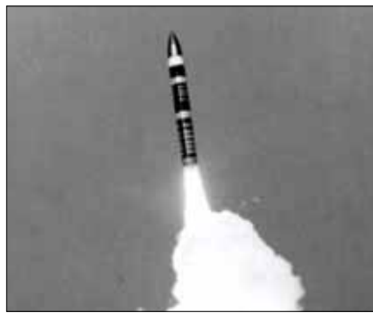
The LGM-118A Peacekeeper, a four-stage intercontinental ballistic missile, became operational near the end of the Cold War. (USAF Photo)
