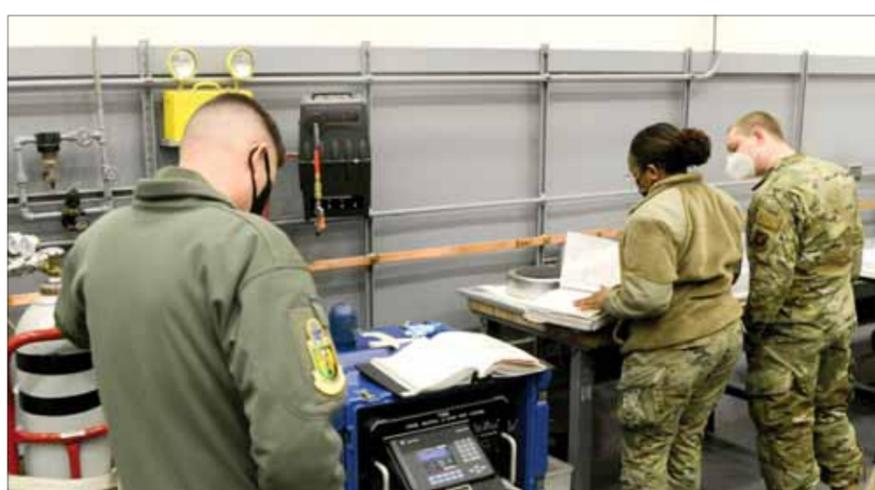
Airmen with the 705th Munitions Squadrons showcase how to operate a T568 on Nov. 22, 2021 at Minot Air Force Base, N.D. The T568 is used to purge and backfill containers for shipping system critical components.
