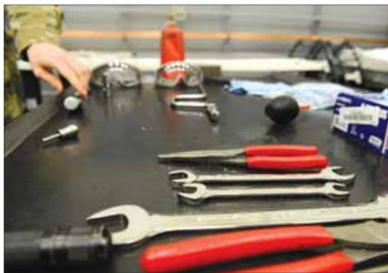
Tools used to operate a T568 by Airmen of the 705th Munitions Squadron are laid out on Nov. 22, 2021 at Minot Air Force Base, N.D. The T568 is used to purge and backfill containers for shipping system critical components.
