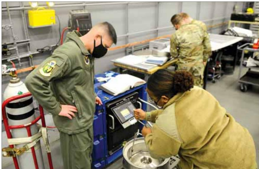
Senior Airman Kenya Cook, Reentry System/Reentry Vehicle Team Chief with the 705th Munitions Squadron, showcases how to operate a T568 on Nov. 22, 2021 at Minot Air Force Base, N.D. The T568 is used to purge and backfill containers for shipping system critical components.
