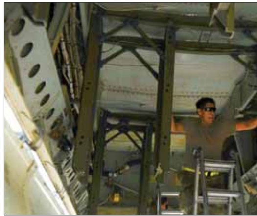
Senior Airman Trenton Garcia and Airman 1st Class Shane Mickolick, 5th Aircraft Maintenance Squadron Weapons Load Crew Members, conduct an operations check in the bomb bay of a B-52H Stratofortress on Dec. 7, 2021, at Edwards Air Force Base, California. The operations check verified that the systems in the B-52 bomb bay will function correctly and are ready to receive the weapons.
