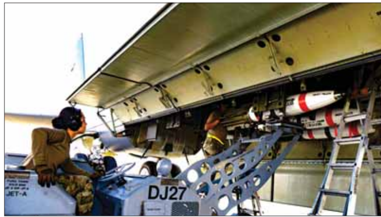
Airman Melissa Lopez (left), Senior Airman Trenton Garcia (center) and Airman 1st Class Shane Mickolick (top right), 5th Aircraft Maintenance Squadron Weapons Load Crew Members, load a mine into the bomb bay of a B-52H Stratofortress during a Bomber Agile Combat Employment exercise on Dec. 7, 2021, at Edwards Air Force Base, California. BACE is part of an initiative to develop and improve our capability to deploy bombers, personnel and equipment to austere or unfamiliar locations on short notice, allowing units to better fulfill future missions in support of Air Force Global Strike Command and Air Force strategic objectives.
