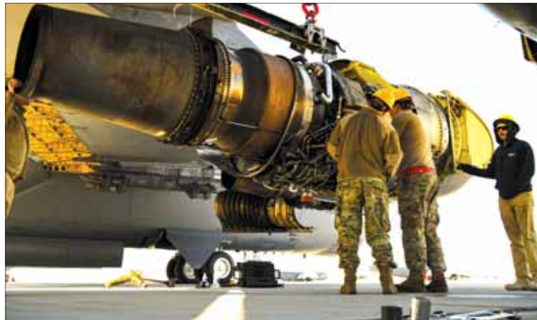
Airmen with the 5th Maintenance Squadron and 99th Civil Engineering Squadron work together to replace a B-52H Stratofortress engine during Red Flag-Nellis 22-1 on Jan. 25, 2022 at Nellis Air Force Base, Nevada. The 5 MXS is one of 32 units from across the U.S. joint forces, United Kingdom (Royal Air Force) and Australia (Royal Australian Air Force) participating in Red Flag-Nellis 22-1.
