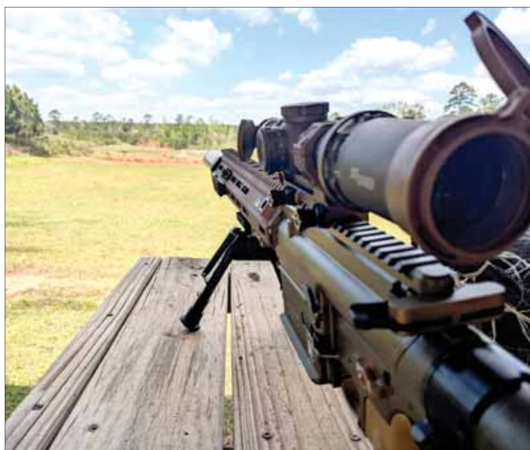
The Squad Designated Marksmanship Rifle is tested on a range at Robins Air Force Base, Ga., April 13, 2022. The SDMR is a semi-automatic, 7.62x51mm caliber rifle designed by Heckler & Koch for missions requiring combat over-watch with precision-fire capability to accurately engage targets up to 600 meters.
