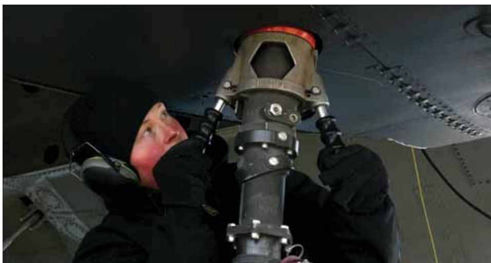
Airman 1st Class Nicole Wiley, 5th Aircraft Maintenance Squadron assistant dedicated crew chief, fuels a B-52H Stratofortress for its next flight on Minot Air Force Base, North Dakota, April 26, 2022. The B-52 uses 3,300 gallons of fuel every hour of flight.
