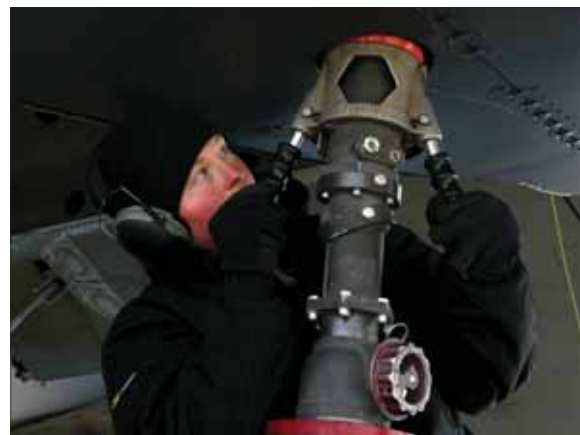
Airman 1st Class Nicole Wiley, 5th Aircraft Maintenance Squadron assistant dedicated crew chief, fuels a B-52H Stratofortress for its next flight on Minot Air Force Base, North Dakota, April 26, 2022. The B-52 uses 3,300 gallons of fuel every hour of flight.
