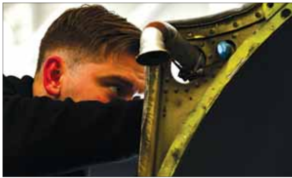
An Airman with the 5th Aircraft Maintenance Squadron runs a de-ice pipe through the frame of a ring cowl on June 6, 2022, at Minot Air Force Base, North Dakota. With de-ice pipes routed within the framework of the ring cowl, ice is prevented from building up on the B-52H engine.
