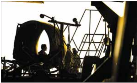
Airmen with the 5th Aircraft Maintenance Squadron prepare to affix a ring cowl to a B-52H Stratofortress engine on June 6, 2022, at Minot Air Force Base, North Dakota. A ring cowl serves to increase air flow into the B-52 engine and optimize pressurization. This helps the engine operate and prevents stalling while the B-52 is still grounded.
