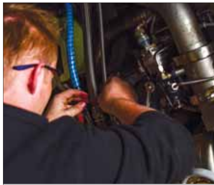
An Airman with the 5th Aircraft Maintenance Squadron runs a de-ice pipe through the frame of a ring cowl on June 6, 2022, at Minot Air Force Base, North Dakota. With de-ice pipes routed within the framework of the ring cowl, ice is prevented from building up on the B-52H engine.
