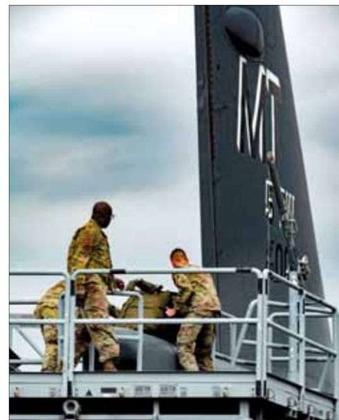
23rd Aircraft Maintenance Unit Airmen from 23rd Expeditionary Bomb Squadron place the drogue parachute back into a B-52H Stratofortress after it was deployed during landing.
