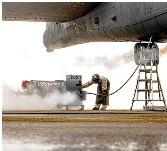
An airman assigned to the 23rd Aircraft Maintenance Unit performs an oxygen refill on a B52-H Stratofortress at Morón Air Base, Spain, Mar. 10, 2023. Strategic bomber missions enhance the readiness and training necessary to respond to any potential crisis or challenge across the globe.
