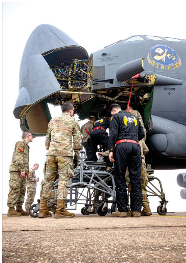
Members of the 23rd Aircraft Maintenance Unit perform a radar antenna swap on a B52-H Stratofortress at Morón Air Base, Spain, Mar. 10, 2023. The U.S. maintains a strong, credible strategic bomber force that enhances the security and stability of Allies and Partners.
