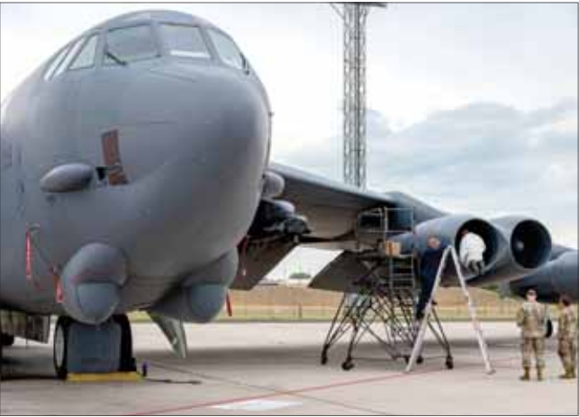
Airmen, assigned to the 5th Aircraft Maintenance Squadron, inspect the intake of a B-52H Stratofortress engine during the Global Strike Challenge at Minot Air Force Base, North Dakota, Aug. 4, 2023. Each of the B-52H Stratofortress' eight engines can produce up to 17,000 pounds of thrust.
