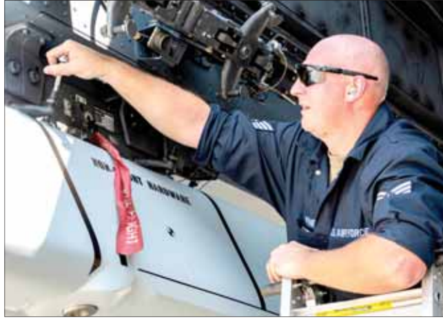
U.S. Air Force Staff Sgt. Lewis Hafner, 5th Aircraft Maintenance Squadron weapons team chief, secures an inert precision guided munition onto the wing pylon of a B-52H Stratofortress at Minot Air Force Base, North Dakota, Aug. 3, 2023. Hafner provided directions to his team throughout the weapons loading process.
