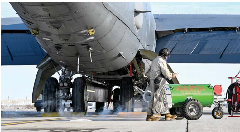
Airman 1st Class Seth Quillen, 5th Aircraft Maintenance Squadron crew chief, looks at his checklist while performing liquid oxygen (LOX) maintenance on a B-52H Stratofortress at Minot Air Force Base, North Dakota, Nov. 2, 2023. Crew chiefs regularly perform LOX maintenance on aircraft to ensure pilots and aircrew have oxygen readily available during flight.
