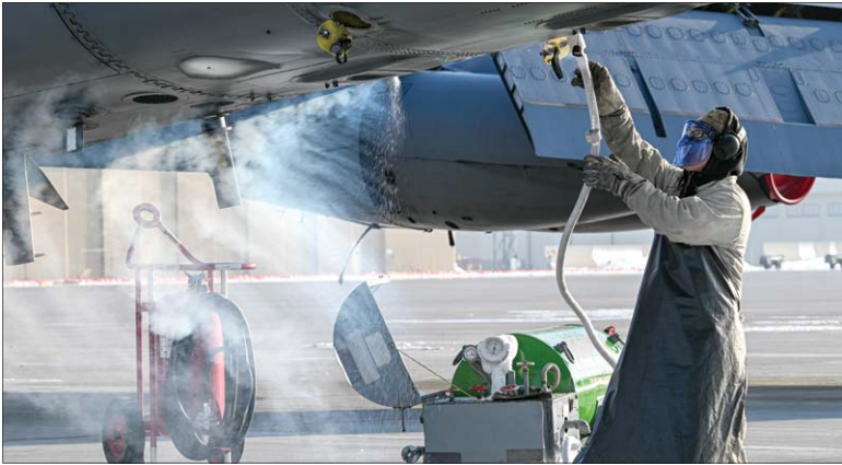
Airman 1st Class Seth Quillen, 5th Aircraft Maintenance Squadron crew chief, connects a liquid oxygen (LOX) hose to a B-52H Stratofortress at Minot Air Force Base, North Dakota, Nov. 2, 2023. The aircraft's systems convert LOX into a gaseous form, providing oxygen to the aircrew during flight.
