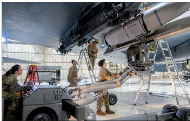
Members of the 5th Aircraft Maintenance Squadron load an inert AGM-158 Joint Air to Surface Standoff Missile (JASSM) onto a B-52H Stratofortress as part of the 2024 annual weapons load competition at Minot Air Force Base, North Dakota, Jan. 19, 2024. Airmen loaded an inert AGM-158 JASSM onto a B-52H Stratofortress as quickly as possible while maintaining all safety precautions.
