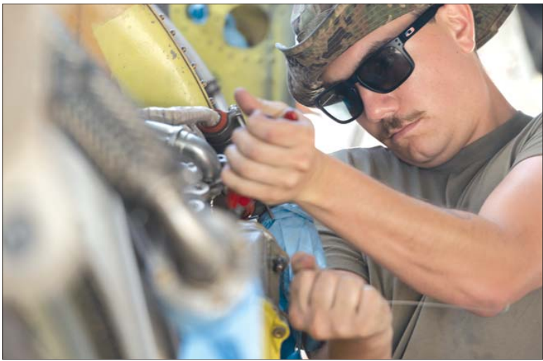
U.S. Air Force Senior Airman Matthew Thibodeau, 5th Aircraft Maintenance Squadron aerospace propulsion technician, replaces an unserviceable constant speed direct oil cooler on a U.S. Air Force B-52H Stratofortress during routine engine maintenance in support of a Bomber Task Force deployment at Andersen Air Force Base, Guam, July 9, 2023. BTF deployments like this enhance the readiness and training necessary to respond to any potential crisis or challenge across the globe.
