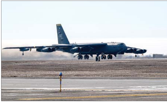
A U.S. Air Force B-52H Stratofortress assigned to the 69th Bomb Squadron, takes off from the runway at Minot Air Force Base, North Dakota, Feb. 28, 2024. Each of the B-52's eight engines is capable of producing up to 17,000 pounds of thrust; allowing it to fly at high subsonic speeds at altitudes of up to 50,000 feet, while carrying a payload of up to 70,000 pounds.
