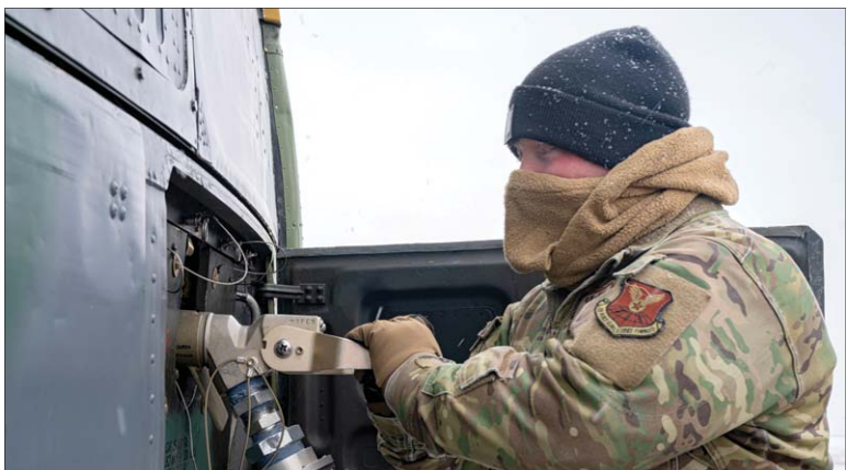
U.S. Air Force Staff Sgt. Michael Norris, 54th Helicopter Squadron (54th HS) evaluator flight engineer, connects a fuel hose to a UH-1N Iroquois at Minot Air Force Base, North Dakota, March 7, 2024. The 54th HS and their fleet of UH-1Ns provide rapid security response capabilities to Minot AFB's missile fields.
