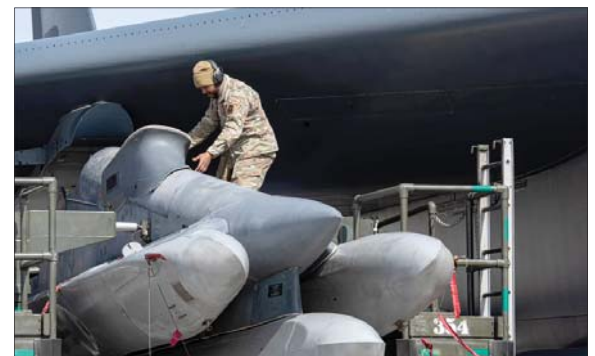
An Airman assigned to the 5th Aircraft Maintenance Group loads AGM-86 air-launched cruise missiles onto a B-52H Stratofortress during Prairie Vigilance 24-3 at Minot Air Force Base, North Dakota, April 6, 2024. Exercises like Prairie Vigilance enable crews to maintain a high state of readiness and proficiency, while validating the always-ready, global strike capability.
