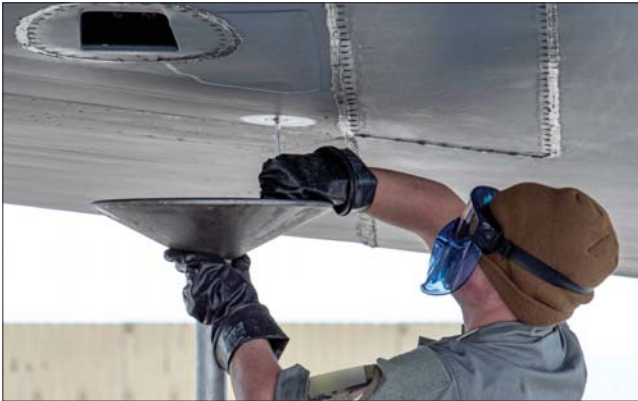
An Airman assigned to the 5th Logistics Readiness Squadron drains fuel from a B-52H Stratofortress during Prairie Vigilance 24-3 at Minot Air Force Base, North Dakota, April 7, 2024. Prairie Vigilance demonstrates the capability, resilience, adaptability, and strength of Team Minot Airmen.
