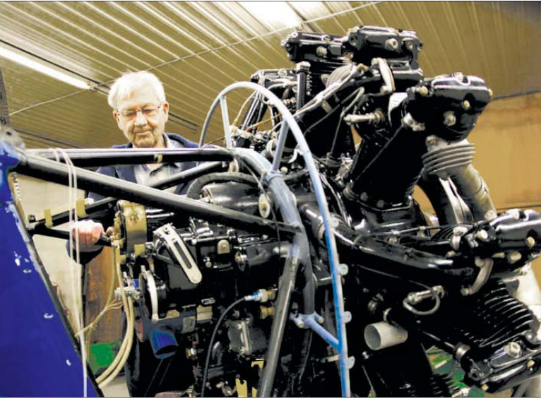
Larry Linrud looking across the newly rebuilt engine. There are 7 cylinders.
