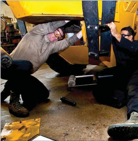
Installing hydraulic lines on a grader vehicle.
