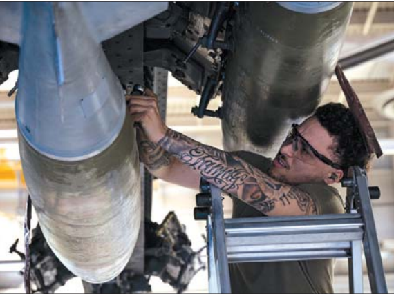
Senior Airman Nicholas Bowden, 69th Bomber Generation Squadron load crew member, secures an inert GBU-31 Joint Direct Attack Munition to a B-52H Stratofortress during the 1st Quarter Weapons Load Competition at Minot Air Force Base, May 2, 2025. Weapons load competitions play a significant role in enhancing mission readiness and strengthening global strike capabilities.
