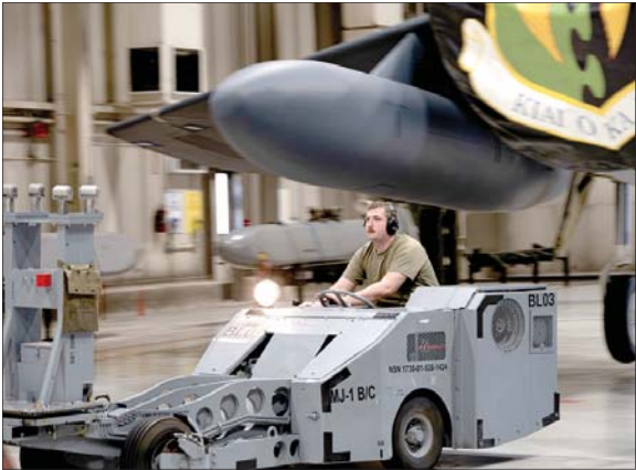
Senior Airman Joshua Boyle, 69th Bomber Generation Squadron load crew member, drives a missile carrier during the 1st Quarter Weapons Load Competition at Minot Air Force Base, May 2, 2025. For the inert munition to be loaded onto the aircraft safely and effectively, the crew must always have precise control over it.
