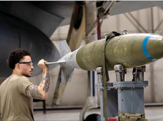
Senior Airman Nicholas Bowden, 69th Bomber Generation Squadron load crew member, prepares to secure an inert GBU-31 Joint Direct Attack Munition to a B-52H Stratofortress during the 1st Quarter Weapons Load Competition at Minot Air Force Base, May 2, 2025. For the inert munition to be loaded onto the aircraft safely and effectively, the crew must always have precise control over it
