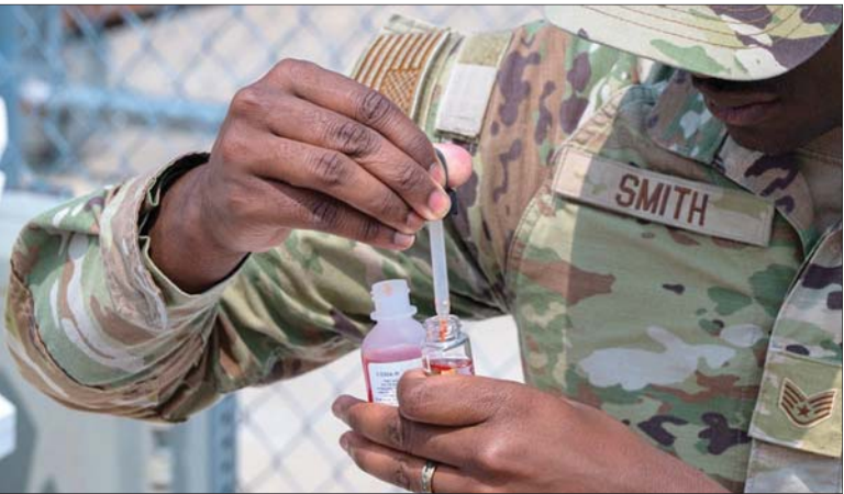
U.S. Air Force Staff Sgt. Jaail Smith, NCOIC of occupational health for the 5th Operational Medical Readiness Squadron (5OMRS), tests the pH balance of the water of the outdoor base pool at Minot Air Force Base, North Dakota, May 30, 2025. Bioenvironmental Engineers play a critical role in protecting the health of the force through air and water quality testing, radiation monitoring, and exposure risk assessments.
