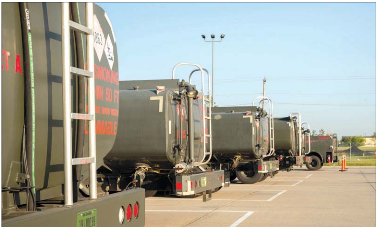
A line of C-300 mobile fuel vehicles are parked at the 5th Logistics Readiness Squadron petroleum, oil and lubricant flight's parking area at Minot Air Force Base, North Dakota, June 24, 2025. A C-300 mobile fuel vehicle is capable of carrying 1,200 gallons of fuel and can dispense 80 gallons of fuel per minute.
