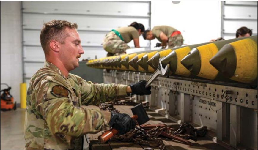
U.S. Air Force Airman 1st Class Zachary O'Shei, 5th Munitions Squadron (5MUNS) crew member, tightens the nose plug on a MK-82 conical munition at Minot Air Force Base, North Dakota, August 4, 2025. 5MUNS will compete in the Air Force Combat Operations Competition designed to test adaptability and technical sharpness.
