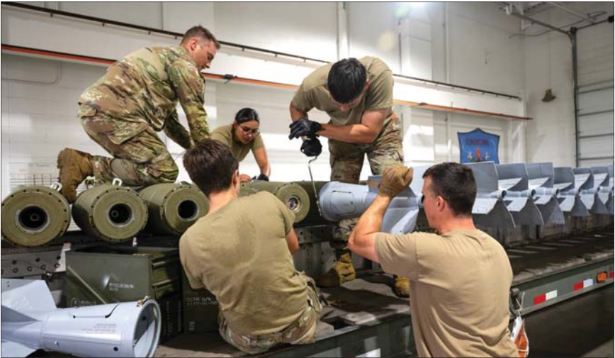
U.S. Air Force Airmen from the 5th Munitions Squadron (5MUNS) build a MK-82 conical munition at Minot Air Force Base, North Dakota, August 4, 2025. 5MUNS built the MK-82 conical in preparation for the Air Force Combat Operations Competition, where they will compete against other munitions squadrons in munition building exercises.
