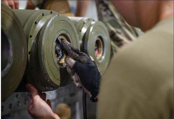
An Airman assigned to the 5th Munitions Squadron (5MUNS) tightens the fuses on the back of a MK-82 conical munition at Minot Air Force Base, North Dakota, August 4, 2025.
