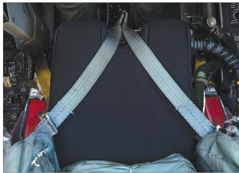
Aircrew from the 49th Test and Evaluation Squadron installed three Kalogon Smart Cushions onboard a U.S. Air Force B-52H Stratofortress for a test flight at Barksdale Air Force Base, La., Nov. 3, 2025. Those overseeing the test hope the smart cushion will decrease pain and injury during long flights and help aircrew recover more quickly between missions—reducing the need for therapy, surgery or rest due to pain.
