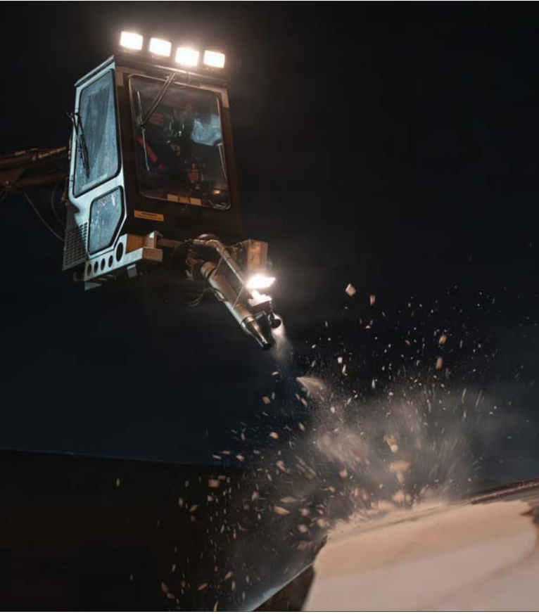
Airman 1st Class Naim Hajji, 23rd Bomb Generation Squadron aerospace propulsion journeyman, de-ices the wing of a B-52H Stratofortress at Minot Air Force Base, North Dakota, Jan. 21, 2026. De-icing ensures the aircraft is safe, effective, and ready for takeoff in winter conditions.
