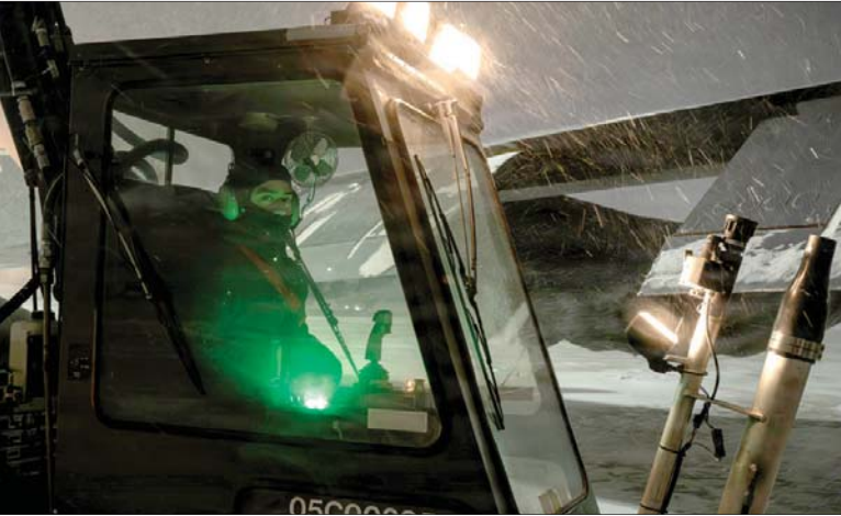
Airman 1st Class Naim Hajji, 23rd Bomb Generation Squadron aerospace propulsion journeyman, prepares to de-ice a B-52H Stratofortress at Minot Air Force Base, North Dakota, Jan. 21, 2026. Aircraft are de-iced to remove ice, snow and frost that has formed on the wings, tail, and control surfaces.
