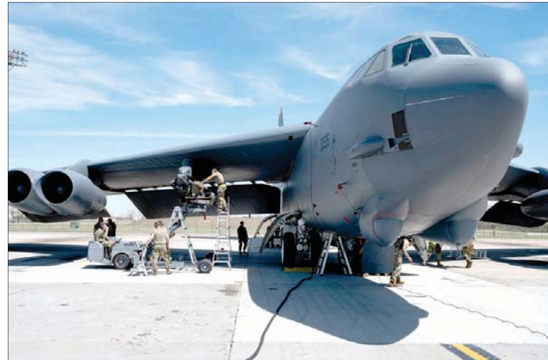
U.S. Airmen assigned to the 5th Maintenance Group load munitions onto a B-52H Stratofortress during Warbird Week at Minot Air Force Base, North Dakota, May 13, 2026. The B-52 is capable of dropping or launching the widest array of weapons in the U.S. inventory.
