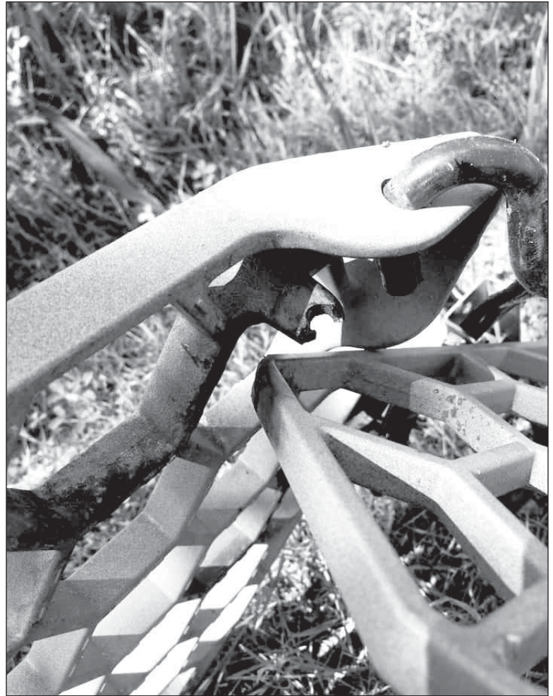
When lightning struck the author's treestand this summer, it melted through solid metal connectors between the foot pad and seat support.
